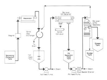
• Sullivan Systems Inc. has designed a new grease recovery system that can handle up to 12,000 pounds per hour of catch basin skimmings for meat and vegetable oil processing facilities. The system uses a De Laval NX decanter for bulk separation and an SAPX solids-ejecting separator for final purification. De Laval says the system reduces pollution problems and cuts cartage costs because skimmings do not have to be transported. Information: Sullivan Systems, Inc., PO Box 158, Tiburon, CA 94920.
